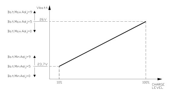
The Battery Charge detection follows this algorithm:
