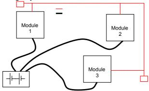
The red lines are can wires.
