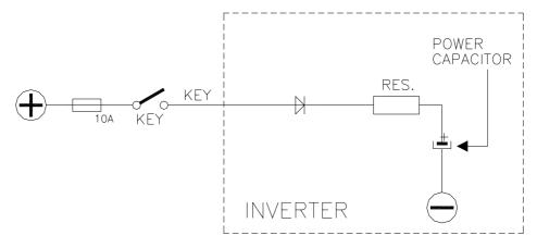
When the key is switched ON, the inverter tries to charge the power capacitors through a power resistance, and check if the capacitor are charged within a timeout. If they do not charge, an alarm is signalled; the main contactor is not closed.
