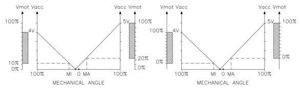
This function looks for and remembers the minimum and maximum potentiometer wiper voltage over the full mechanical range of the pedal. It enables compensation for non symmetry of the mechanical system between directions. The operation is performed by operating the pedal after entering the PROGRAM VACC function.
